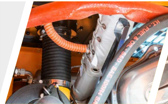
Heavy-duty filtration system (ejector)
