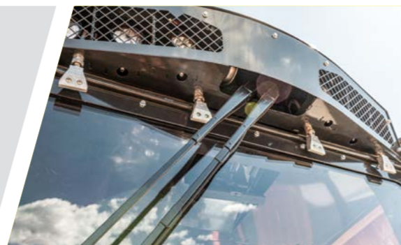
Air window cleaning system
