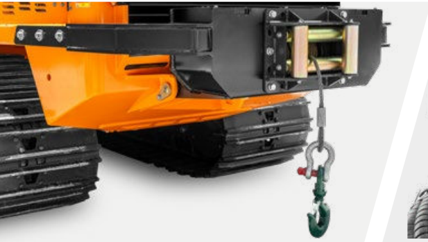
Rear winch with 13-t traction force
