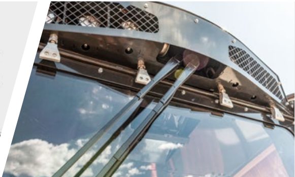
Air window cleaning system
