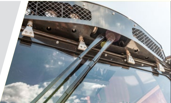
Air window cleaning system
