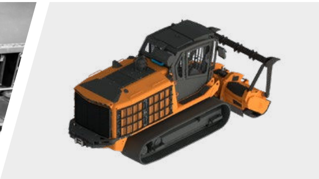
Forestry protection kit (cabin side window grilles + engine compartment door protectors)
