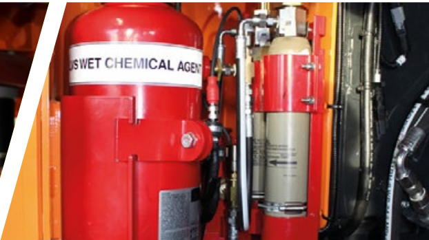
Automatic fire-extinguishing system
