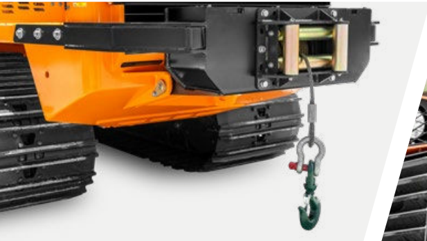
Rear winch with 6-t traction force
