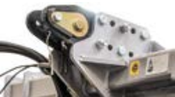
Adjustable extended 3 point hitch fits perfectly with any kind of tractor
