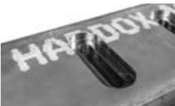
Adjustable Hardox® counter-blade effectively control the final product size
